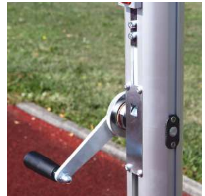
crank mechanism with quick brake to secure crossbar support against uncontrolled movements
