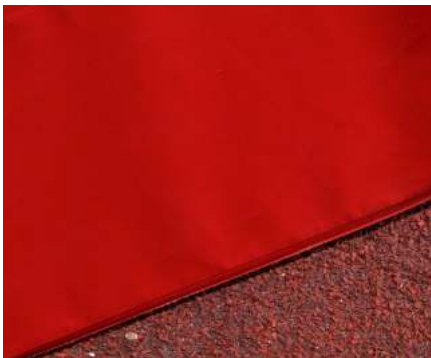
PVC covering made of polyester with two vinyl layers
